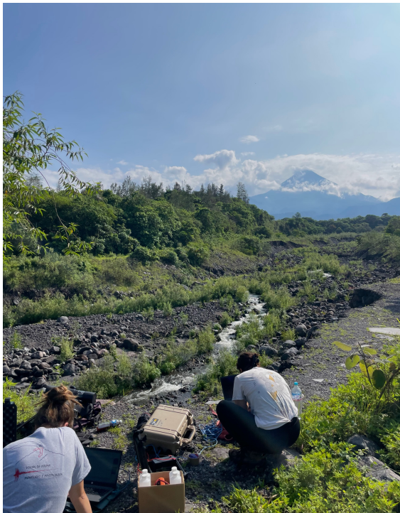
Fieldwork taking SO 2 measurements of the volcano (seen in the distance in the left photo). A direct, cloudless view of the summit is required, so conditions here were sub-optimal. Right: setting up instruments (ScanDOAS and 'SO 2 camera', which have different ways of measuring SO 2 ).
