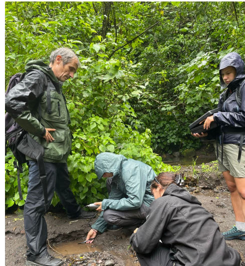
Spring sample collection. Left: The rainy trek to the site at the base of the volcano, which is hidden behind the clouds. Right: Collecting water samples from the spring (muddy puddle, at first appearance). We measured temperature and pH in-situ, and sent samples for chemical analysis.
