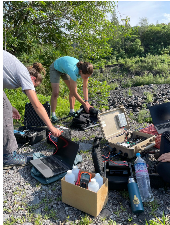
Fieldwork taking SO 2 measurements of the volcano (seen in the distance in the left photo). A direct, cloudless view of the summit is required, so conditions here were sub-optimal. Right: setting up instruments (ScanDOAS and 'SO 2 camera', which have different ways of measuring SO 2 ).
